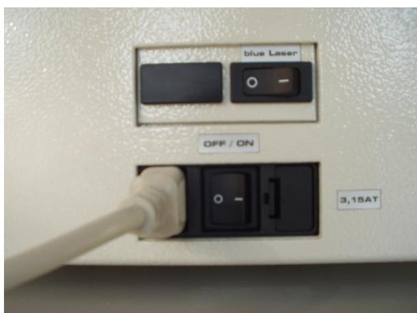
Fig. 10: Power connection and laser switch on the left side of the CyFlow® space.
