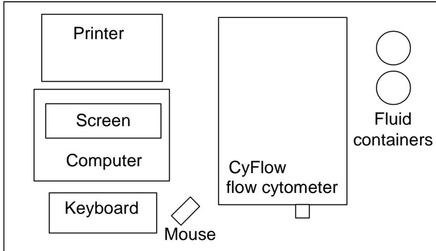
Fig. 7: Recommended placement of CyFlow<sup>®</sup> space components
