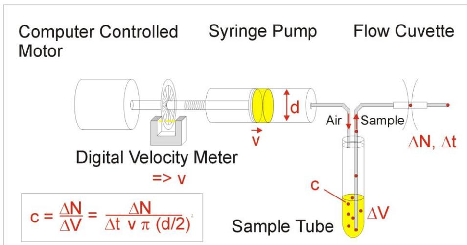
Fig. 6: Sample Transporting System of the CyFlow® space.
