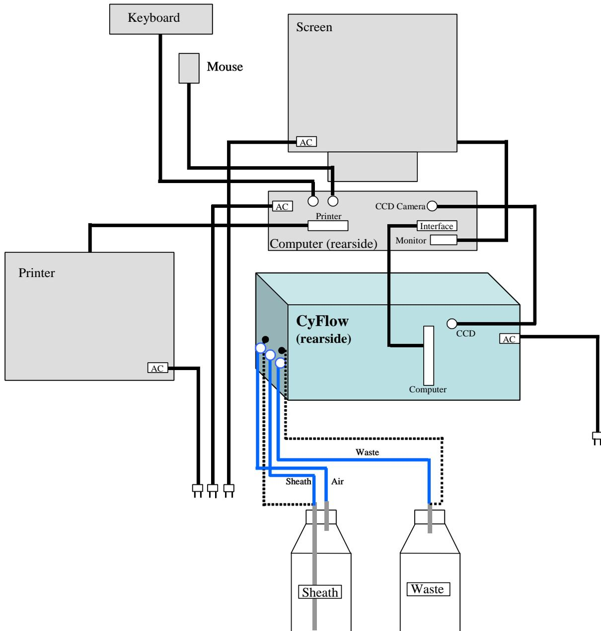
Fig. 8: Instrument Setup and periphery (CyFlow<sup>®</sup> space shown from the rear side).
