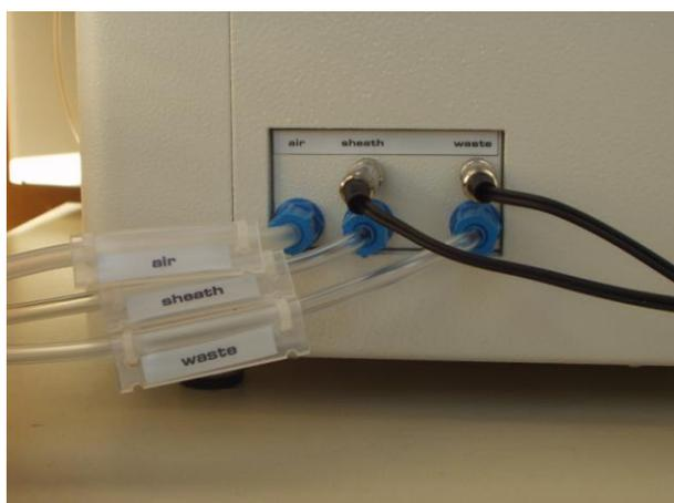
Fig. 11: Tube connections for sheath and waste containers and cable connections for the fluid level sensors on the right side of the CyFlow® space.
