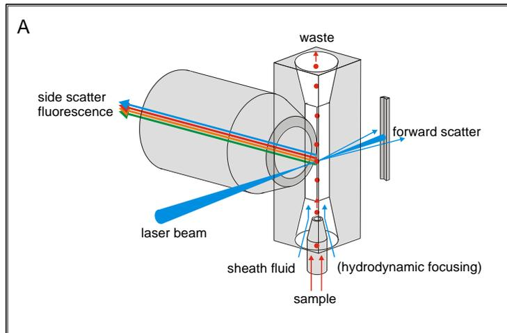
Fig. 3: Optical geometry at the flow cuvette (schematics).
