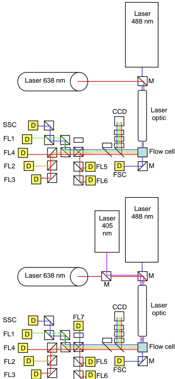
Fig. 2: Exemplary demonstration of the optical bench of a CyFlow® space with 2 lasers and 8 parameters (top) and 3 lasers and 9 parameters (bottom). Other laser light sources and parameter allocations possible. D detector (photo multiplier)
