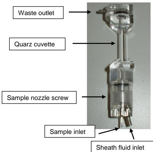
Fig. 12: Flow cuvette with sample, sheath fluid and waste connections.
