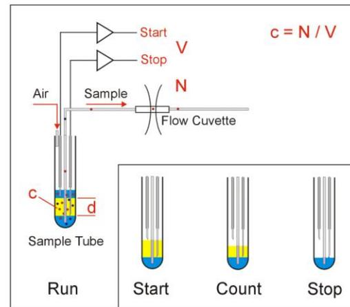
Fig. 1: True Volumetric Absolute Counting by the Electrode Principle.
